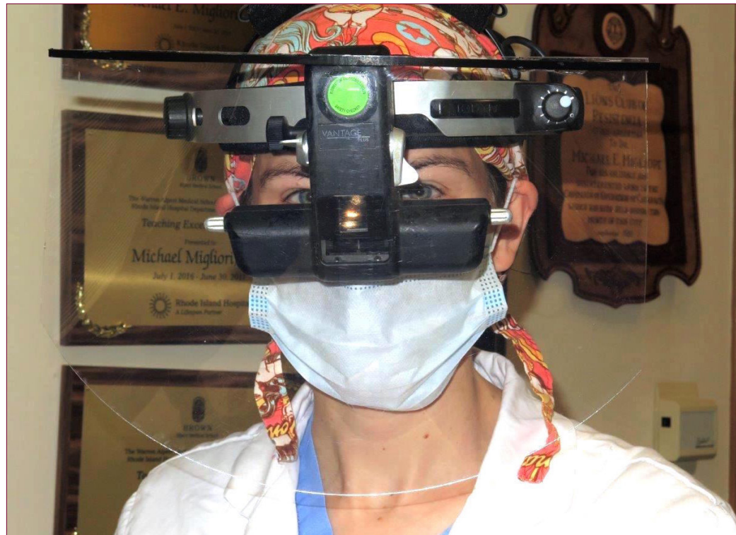
Pediatric Ophthalmologist Melissa Simon, MD , wearing a clip-on shield created by Dr. Woo's 3D Printing Lab, designed to give full-face protection and fit over a binocular indirect ophthalmoscope.
